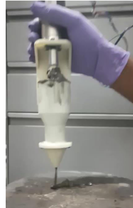
Extruder prototype for cement paste printing
